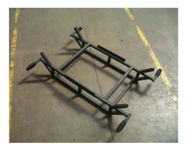
This is an example of a cradle built by a competitor on Series 4. It enables the Robot to run with wheels off the bench or floor and also allows the Robot to be moved easily and safely.
