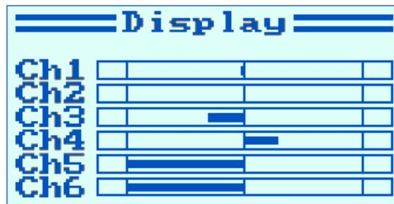
Move each stick/switch/knob to verify the effects of Channel Reversing, End Points, Auxiliary Channel Positions, Dual Rates, Switch Assignments, and Mixes.
