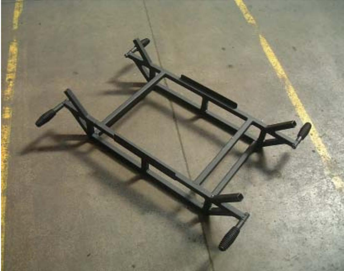
**This is an example of a cradle built by a competitor on Series 4. It enables the Robot to run with wheels off the bench or floor and also allows the Robot to be moved easily and safely.**
